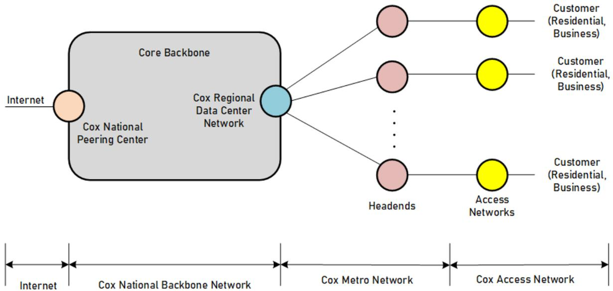
**Figure 3 – Cox Communication High Level Network Architecture**
