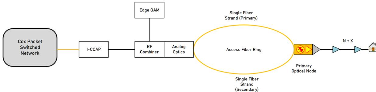
**Figure 2 – Cox Communication Legacy Cable Network Infrastructure**
