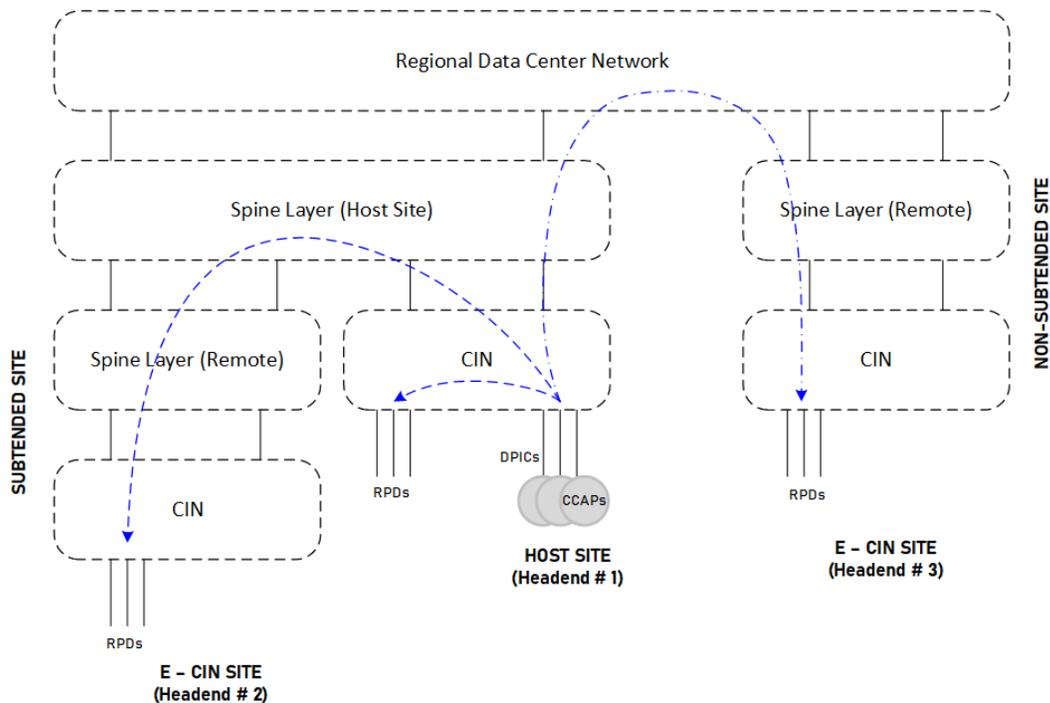
Figure 6 – Cox Communication High-level E – CIN Topology
