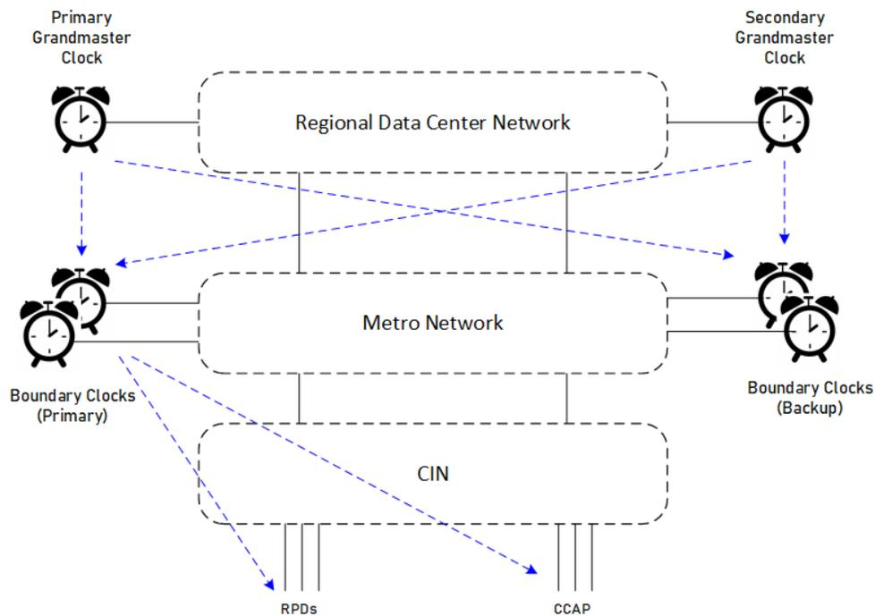
Figure 7 – Cox Communication High-level PTP Architecture
