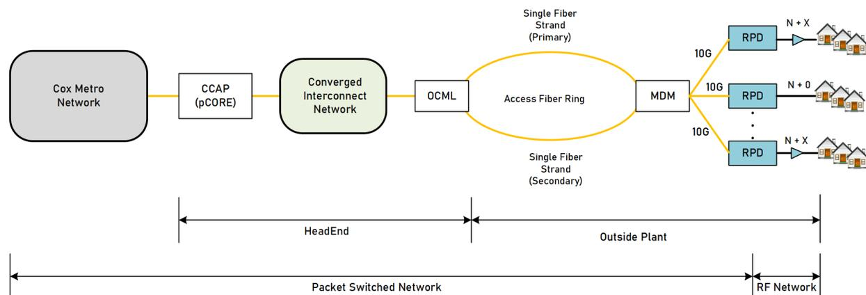
**Figure 4 – Cox Communication High Level DAA Network Topology**
