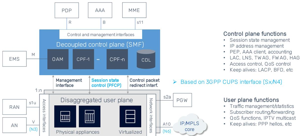
**Figure 4. Disaggregated multi-access edge gateway with CUPS**
