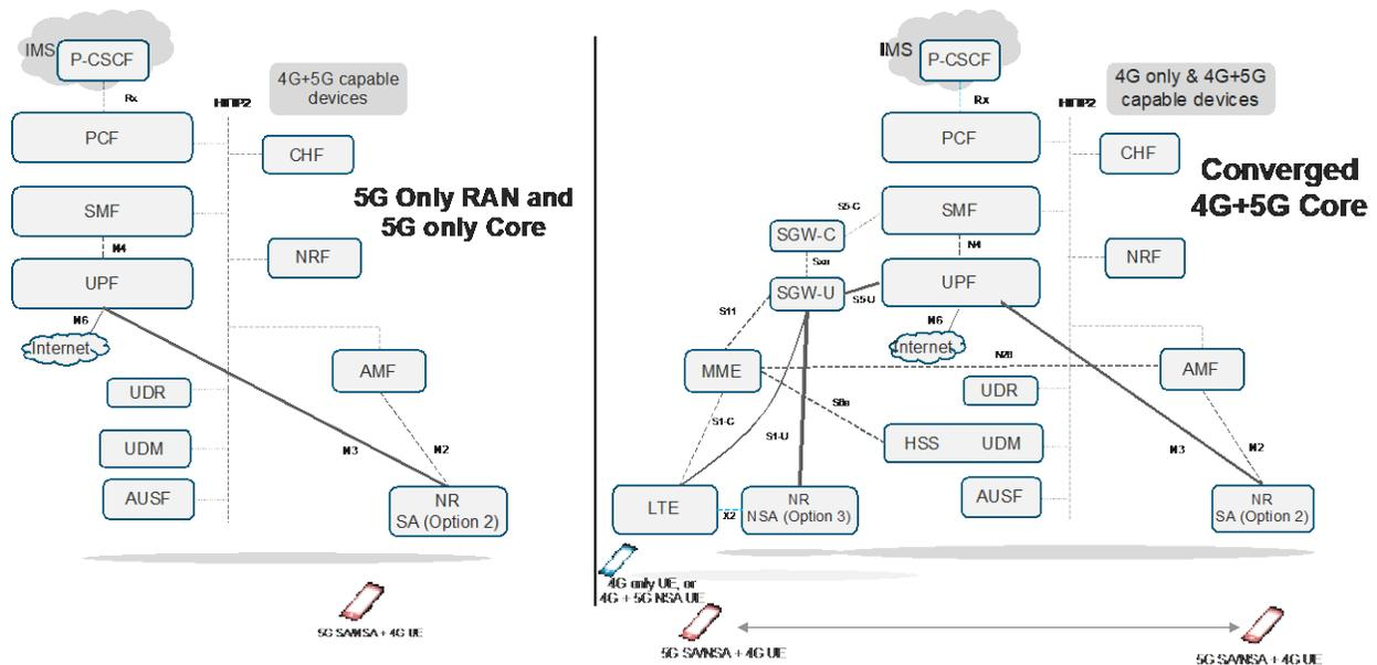
**Figure 7: Converged 4G+5G Core architecture vs. 5G SA architecture**
