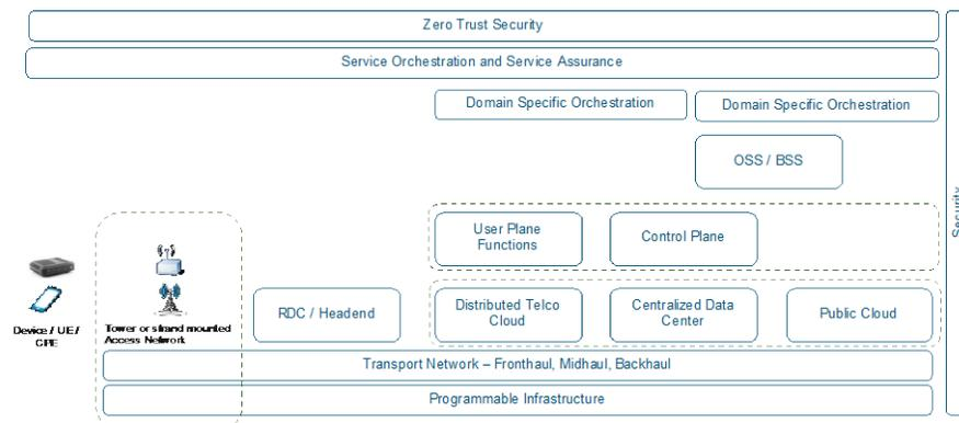
**Figure 1: Different Domains of a typical 5G network**
