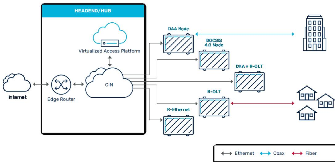
**Figure 8 – Converged Multi-services Cable Access Network**
