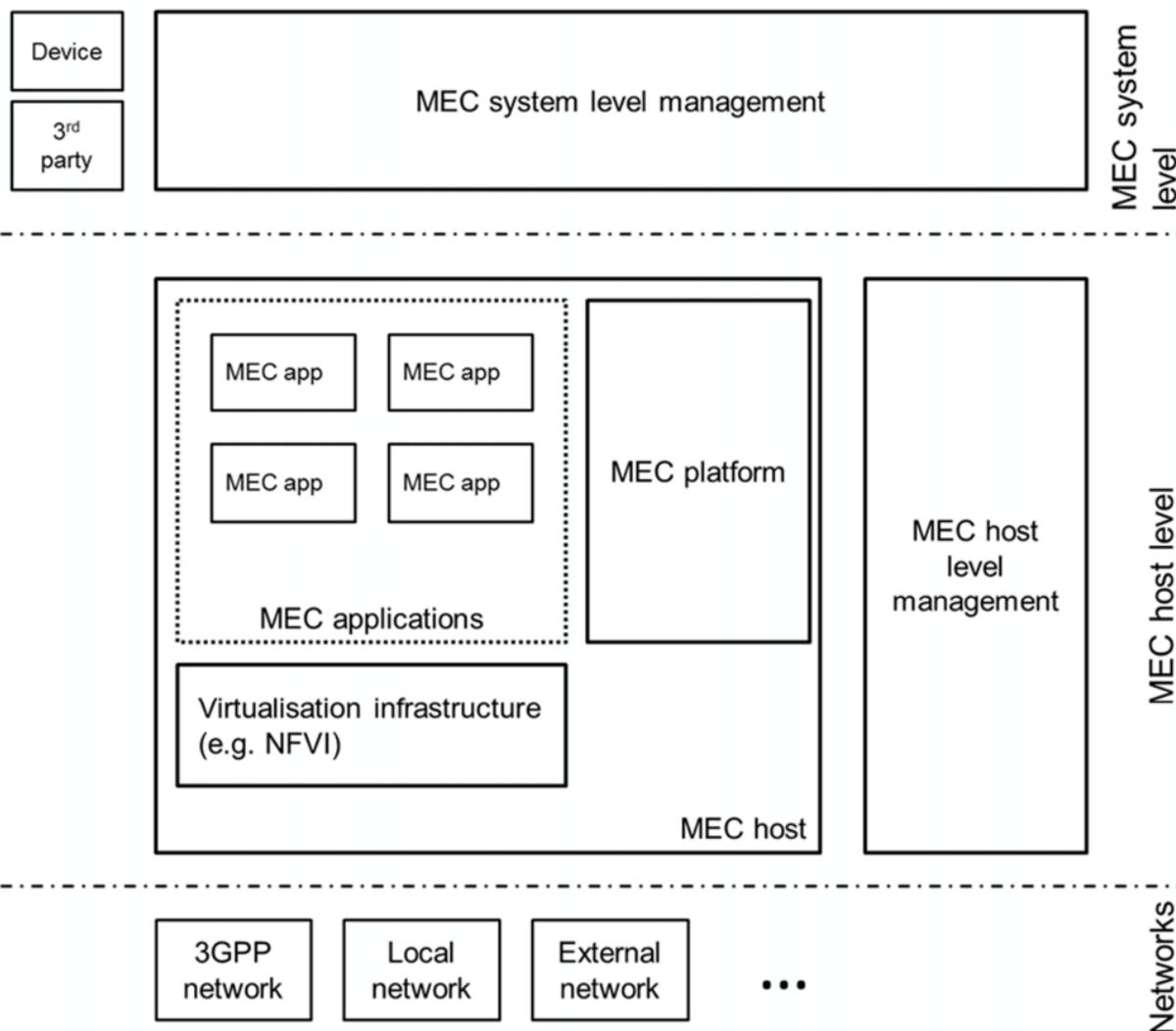
Figure 5 – ETSI Definition of Multi-access Edge Computing Framework [7]
