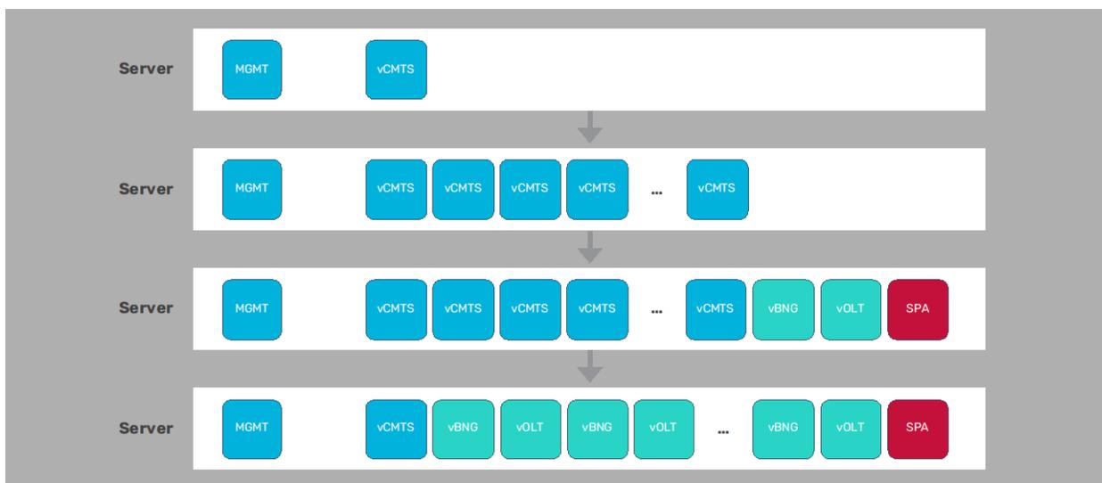
**Figure 4 – Horizontal Scaling of CNFs on a Converged Access Platform**
